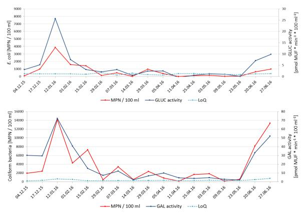
Figure 1: Results of the analysed river water samples taken from December 2015 – June 2016. The enzymatic activity in the samples was measured with BACTcontrol and compared to the cultural method using Colilert. Above: GLUC activity and detected MPN of *E. coli* per 100 ml. Below: GAL activity and detected MPN of coliform bacteria per 100 ml. The respective LoQ was calculated for each measurement by BACTcontrol.
