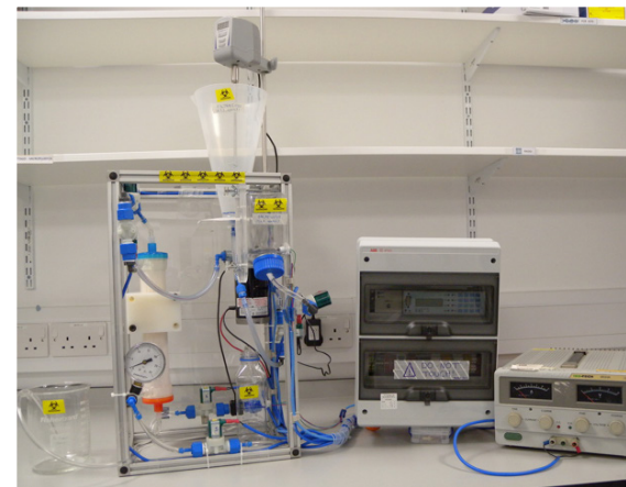
Figure 1 The automated sampling and filtration system for the detection of parasites
