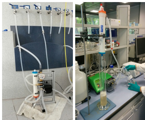
Figure 3 Pictures of different procedures during sampling campaigns. Left picture: On-site filtration in Germany, Right picture: Filter elution in the laboratory at Aigües de Barcelona
